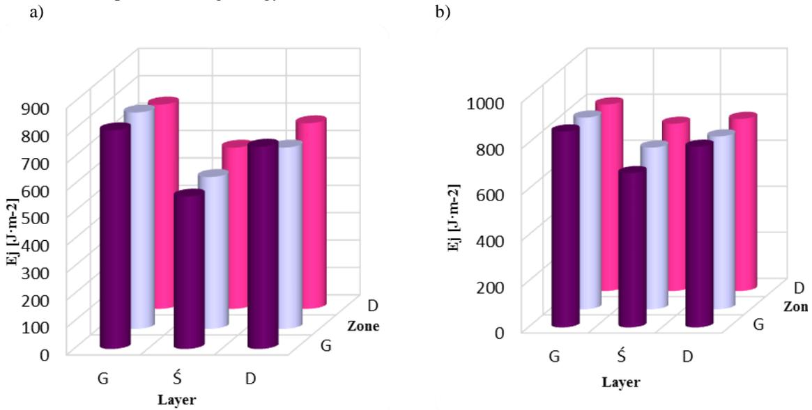
**Fig. 11.** Dependence of specific cutting energy of the black radish parenchyma at knife wedge angle  $\beta = 12,5^\circ$  on the place of sampling at: a) a longitudinal b) transverse fibers orientation
