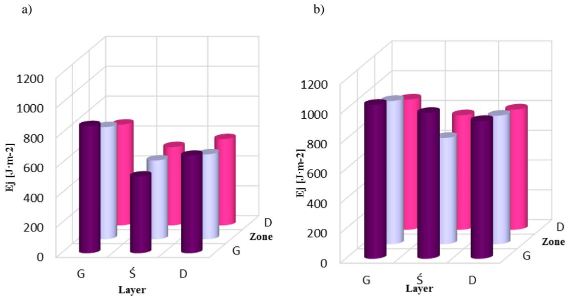
**Fig. 13.** Dependence of specific cutting energy of the black radish parenchyma at knife wedge angle  $\beta = 15^\circ$  on the place of sampling at: a) longitudinal b) transverse fibers orientation
