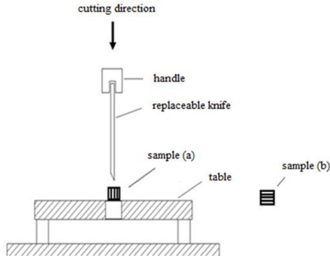
**Fig. 2.** Scheme of equipment for cutting
