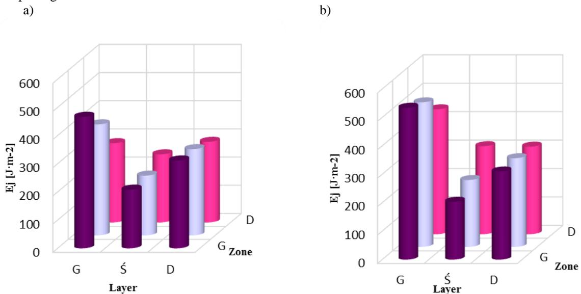
**Fig. 3.** Dependence of specific cutting energy of the black radish parenchyma at knife wedge angle  $\beta = 2.5^\circ$  on the place of sampling at a) longitudinal b) transverse fibers orientation
