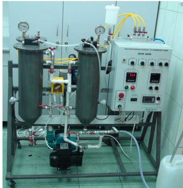
**Fig. 2.** Reactor GW 200 for production of Biodiesel FAME (SME)
