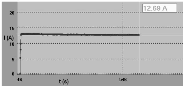
**Fig. 6.** Waveform of the current powering the mill inductor during the grinding of material (time 300 sec.)
