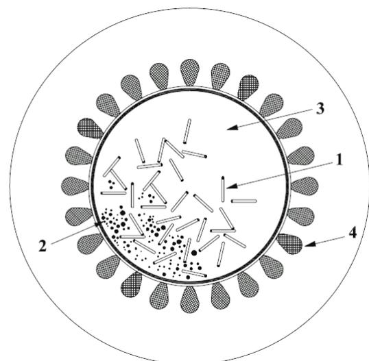
**Fig. 1.** Electromagnetic mill with non-salient poles: 1 – grinding aids, 2 – ground material, 3 – working chamber, 4 – winding in the grooves
