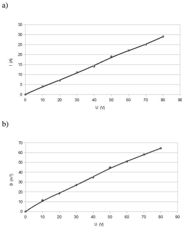
**Fig. 3.** Current intensity (a) and magnetic induction (b) depending on the supply voltage
