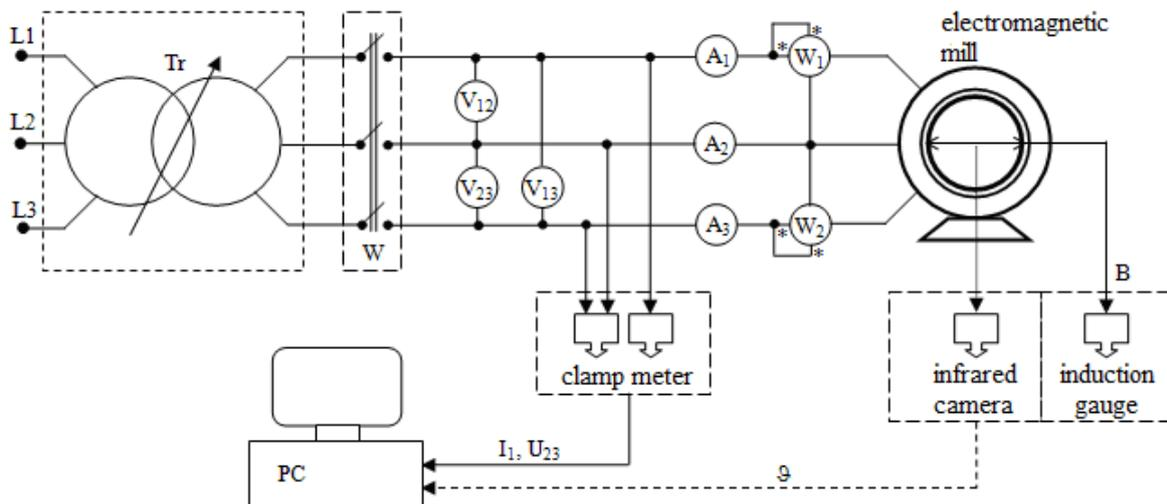
**Fig. 2.** The measuring system of the electromagnetic mill: L1, L2, L3 – different phases of the power supply; Tr – autotransformer; V12, V23, V13 – voltmeters (phase-to-phase voltage); A1, A2, A3 – ammeters (current phase), W1, W2 – watt-meters (power consumed by the mill); PC – computer
