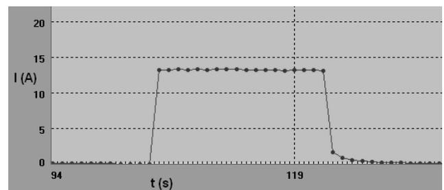
**Fig. 5.** Waveform of the current powering the mill inductor during the switching on and off of the supply voltage
