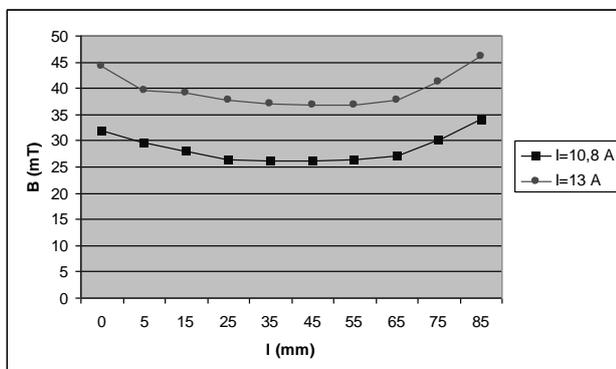
**Fig. 7.** Characteristics of the distribution of magnetic induction within the process chamber of the mill with the inductor windings delta-coupled
