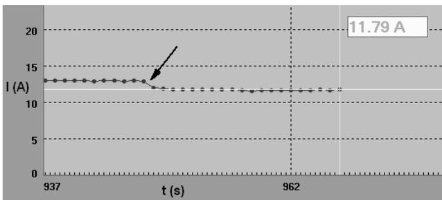
**Fig. 4.** Waveform of the current powering the mill inductor during the filling of the grinding media
