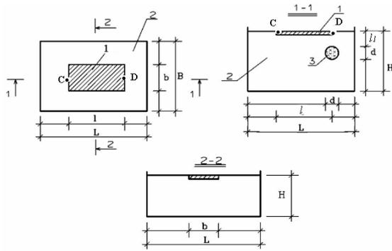
**Fig. 5.** Scheme of the "Clay tray – Base - a foundation."
