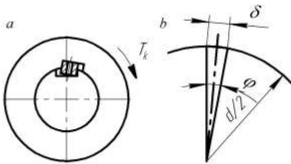
**Fig. 7.** Scheme of the resilient parallel key deformation:
