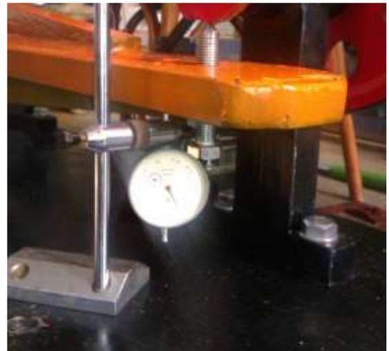
**Fig. 9.** Measuring of the lever angular displacement by the dial indicator
