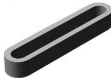
**Fig. 1.** Resilient parallel key with the equidistant cavity
