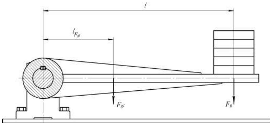
**Fig. 5.** Stand with equipment for the research of static loadings due to weight
