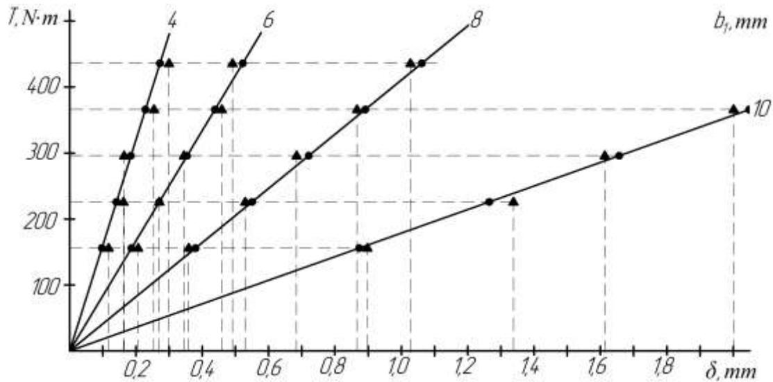
Fig. 10. Graphical dependences between torque and key deformation: ● – theoretical; ▲ – experimental
