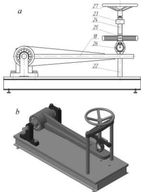
**Fig. 3.** Stand with equipment for the research of statics and calibration of the measure sensor:
