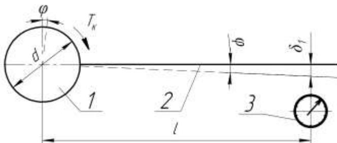
**Fig. 8.** Scheme for definition of the resilient key deformation that is the result of lever angular displacement
