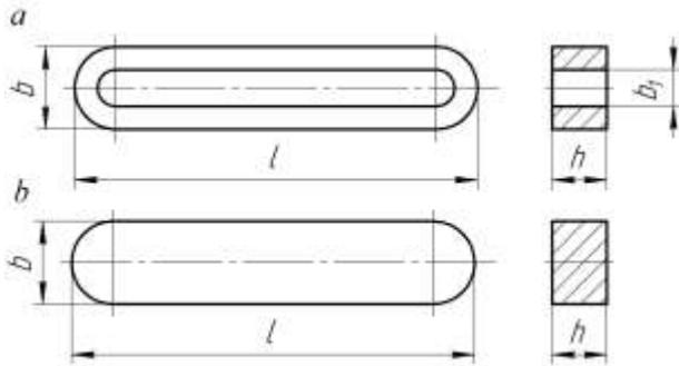
**Fig. 4.** Parallel keys: a – resilient; b – rigid
