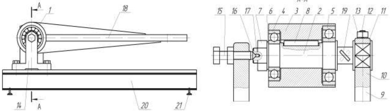
**Fig. 2.** Scheme of the basis of stand for the experimental research of the parallel keyed connections
